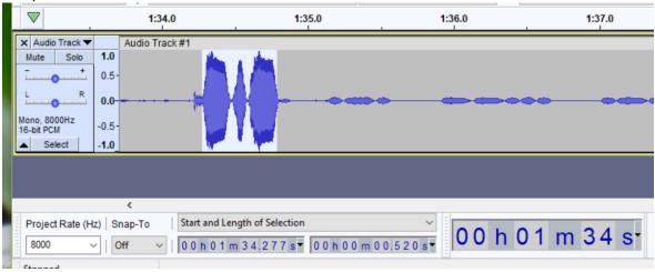
How fast is someone sending? Match to local keyer, or measure some dits... Checking a bug dit ratio with a noisy signal.
