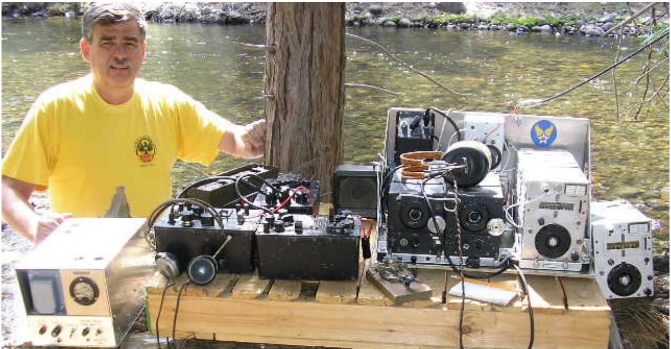
N6CC during "Vintage Field Day" circa 2012. Running CW with the GRC-109 and a Command Set with 80 and 40 meter systems powered by an AC supply with gas generator. Stanislaus River campsite CA.
