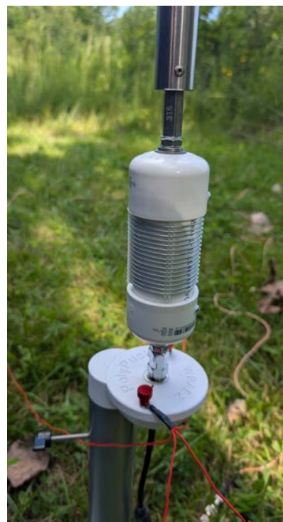
Left: PickupPolyPuck in the hitch, solid enough for a 25-foot whip. Right: Flagpole Base PolyPuck with a base-loaded coil.
