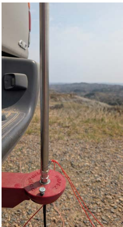
Left: PickupPolyPuck in the hitch, solid enough for a 25-foot whip. Right: Flagpole Base PolyPuck with a base-loaded coil.
