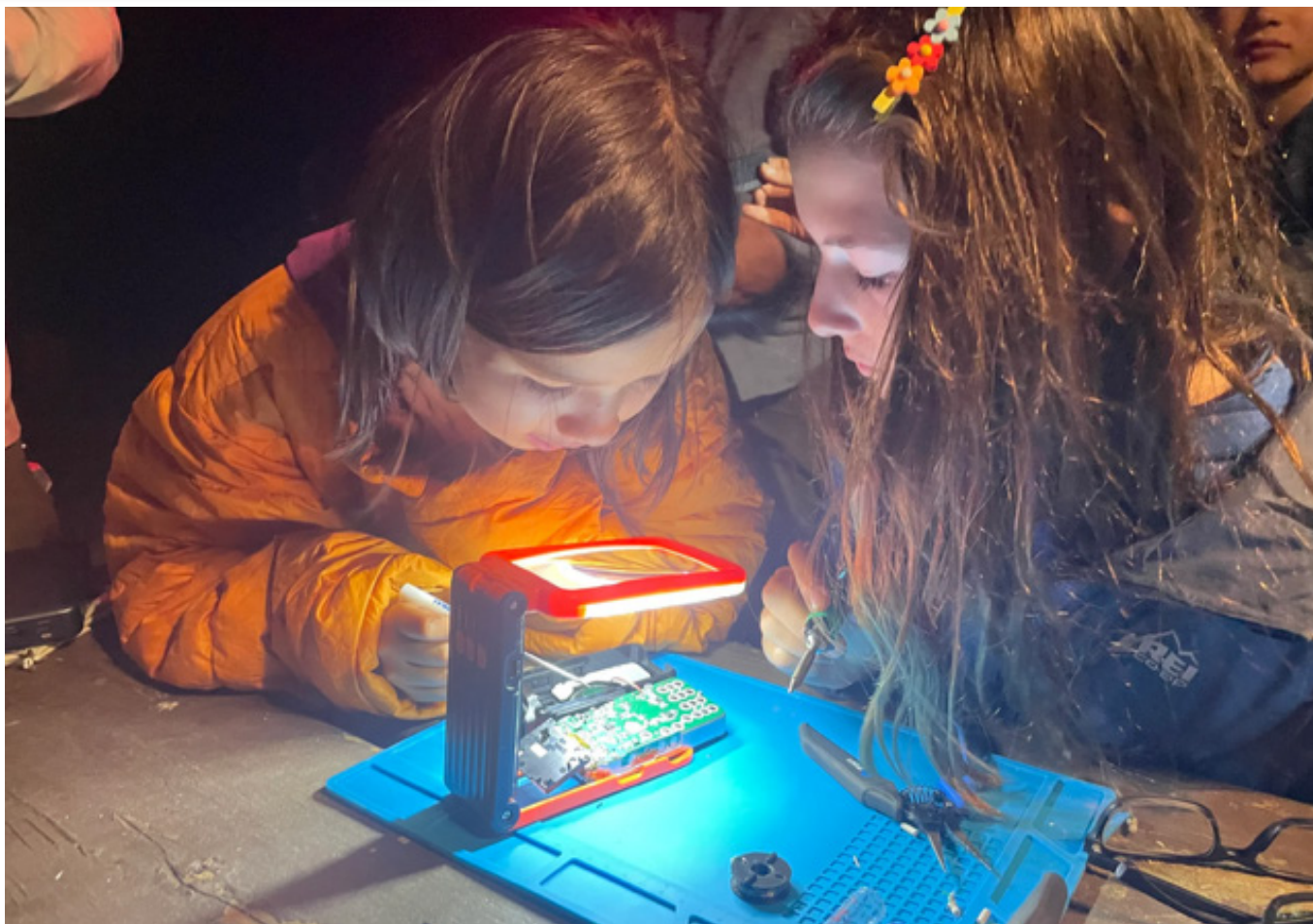
Alice, who holds a Technician-Class license, modifies a Quansheng radio to do CW on 2M, adding the 20K and 10K resistors in the key circuit. Working with Surface mount technology, no less! (Photo by Bob Cady, W7JNM)
