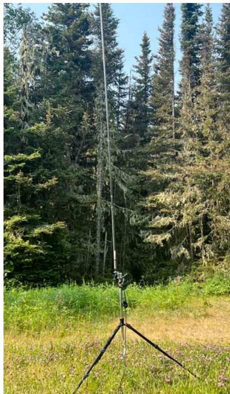
Performer antenna 1/4 wave vertical with 25' whip and 2 resonant elevated radials
